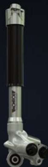
2023 Mercedes-Benz AMG C63 S E Performance plug-in hybrid Monroe Intelligent Suspension CVSA2 electronic dampers
