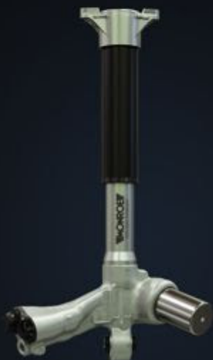
2023 Mercedes-Benz AMG C63 S E Performance plug-in hybrid Monroe Intelligent Suspension CVSA2 electronic dampers
